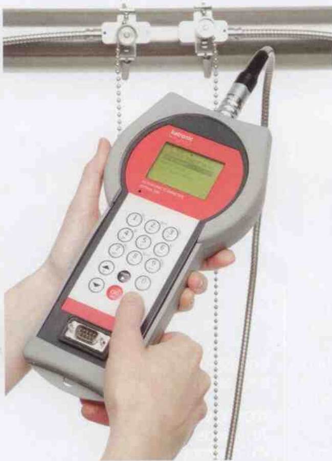
Figure 3. Clamp-on flowmeters provide the user with the unique functionality of a genuinely portable measurement, seen here the KATflow 200 and transducers in operation.
