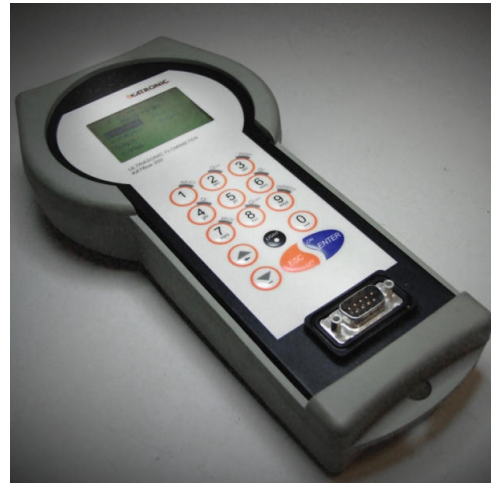
Hand-held ultrasonic clamp-on flowmeter KATflow 200 with one flow channel.
