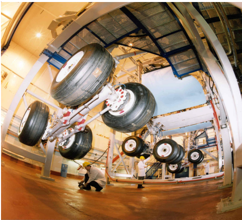
Airbus UK landing gear test rig. Clamp-on sensors were installed to measure the flow of the hydraulic oil in the landing gears.
